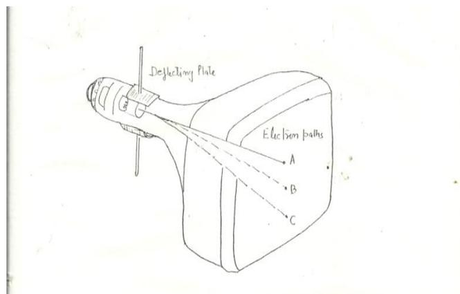
Fig 9 electron motion in CRO
