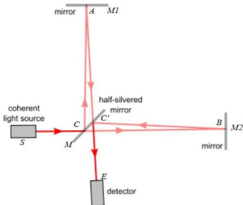
**Fig 3** A Michelson interferometer is used to detect gravitational waves. As a wave passes, each of the arms of the interferometer changes length by different amounts. Wikimedia Commons
